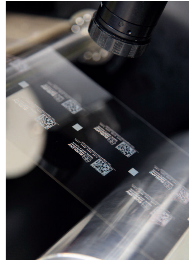
Validus Technologies develops security marks for brand protection using inkjet technology. Photo: Bureau Lorient Communicatie
