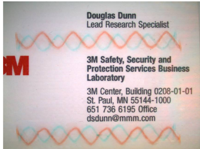
From figure 12 of the paper presented by Douglas Dunn of 3M Safety, Security, & Protection Services Laboratory (USA). Transparent floating image film containing red floating and green sinking sine waves.
